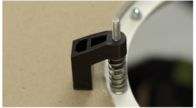
Insert the frame and twist the mounting feet out. Screw down the mounting feet to create the right amount of tension.
