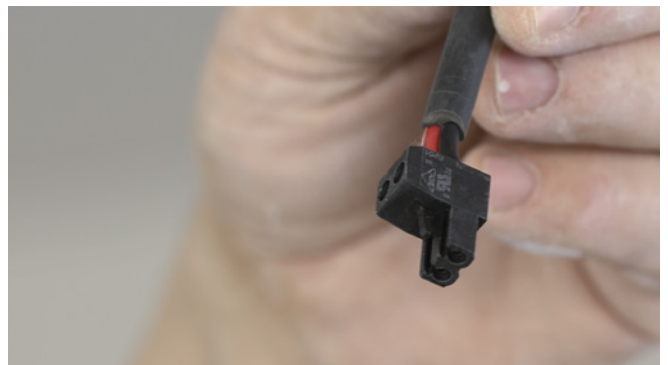
Isolate the speaker cable and connect the system terminals. Make sure the polarity is correct. + is to the right of the terminal.
