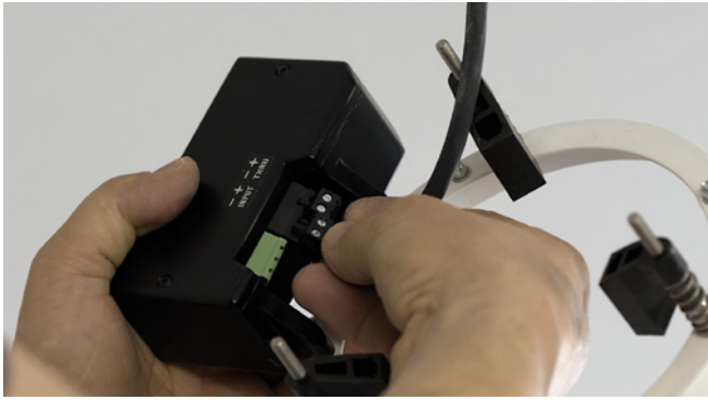
Insert terminal at input of crossover.
